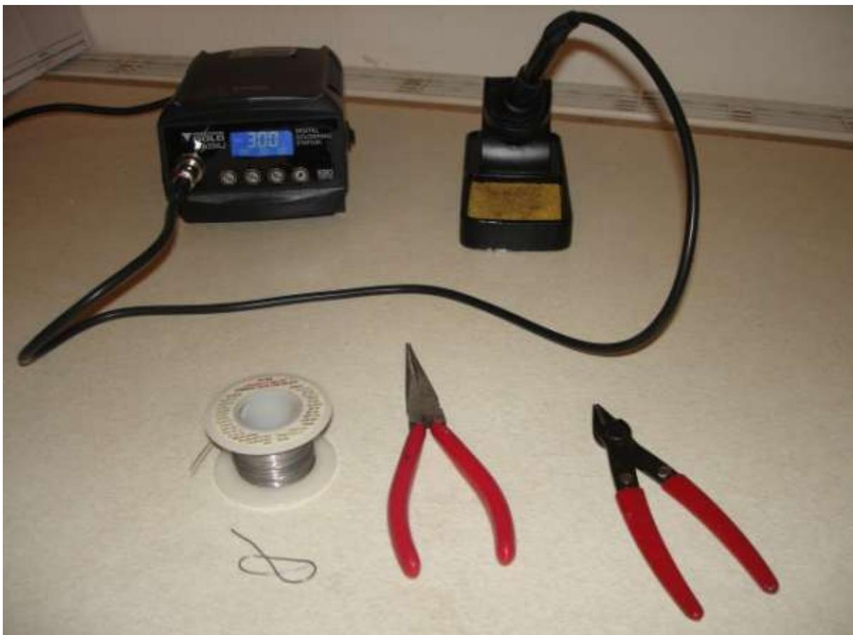
a soldering iron, solder, pliers and a pair of side cutters. In addition, a heat shunt, magnifying glass and multi-meter will make your life much easier.
