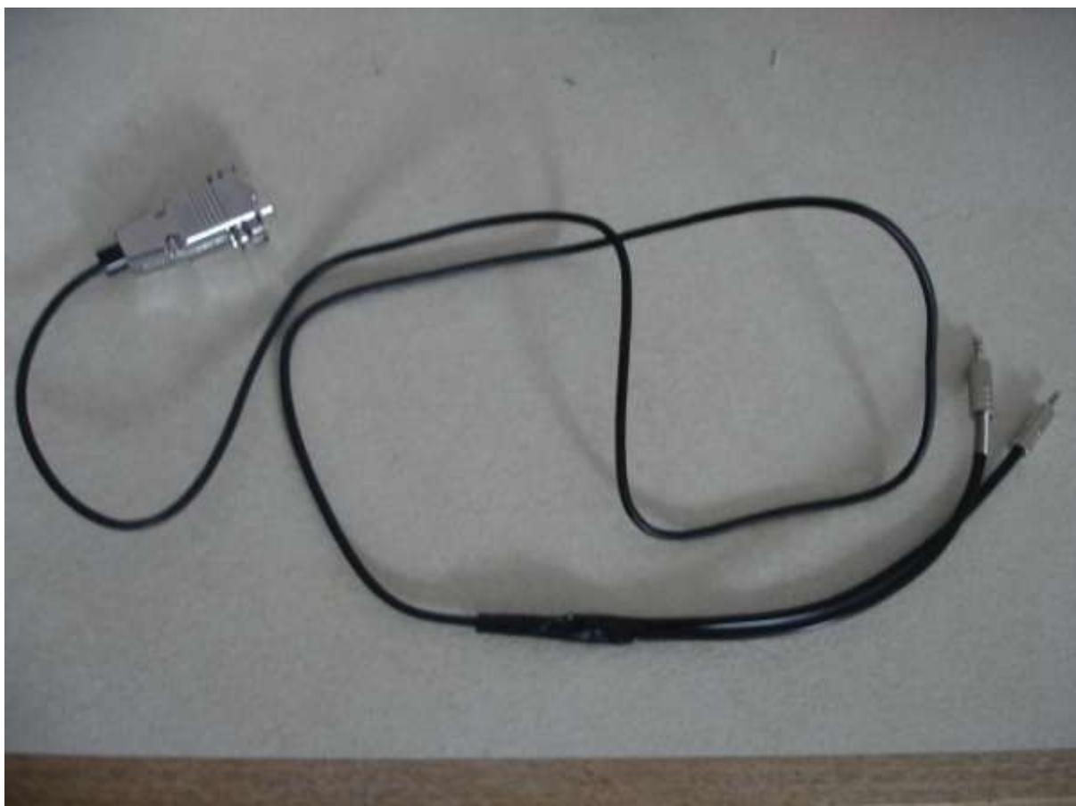
Finally, some tape, heat-shrink sleeve or potting compound secures the tinfoil and improves the cable's mechanical strength (I used tape for speed).
