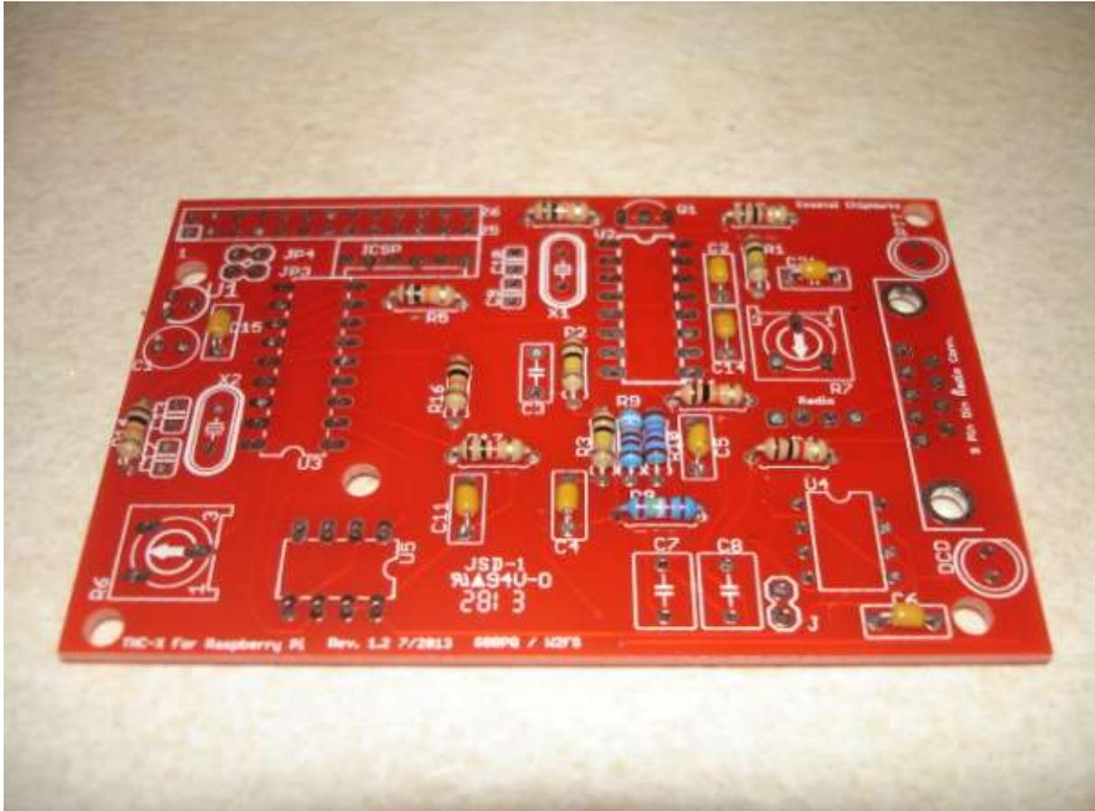
As you can see above, some of the resistors supplied are the blue bodied style which makes the colour bands hard to read. If you have good eyesight then you should be fine but using a multi-meter to check their values is a wire precaution.
