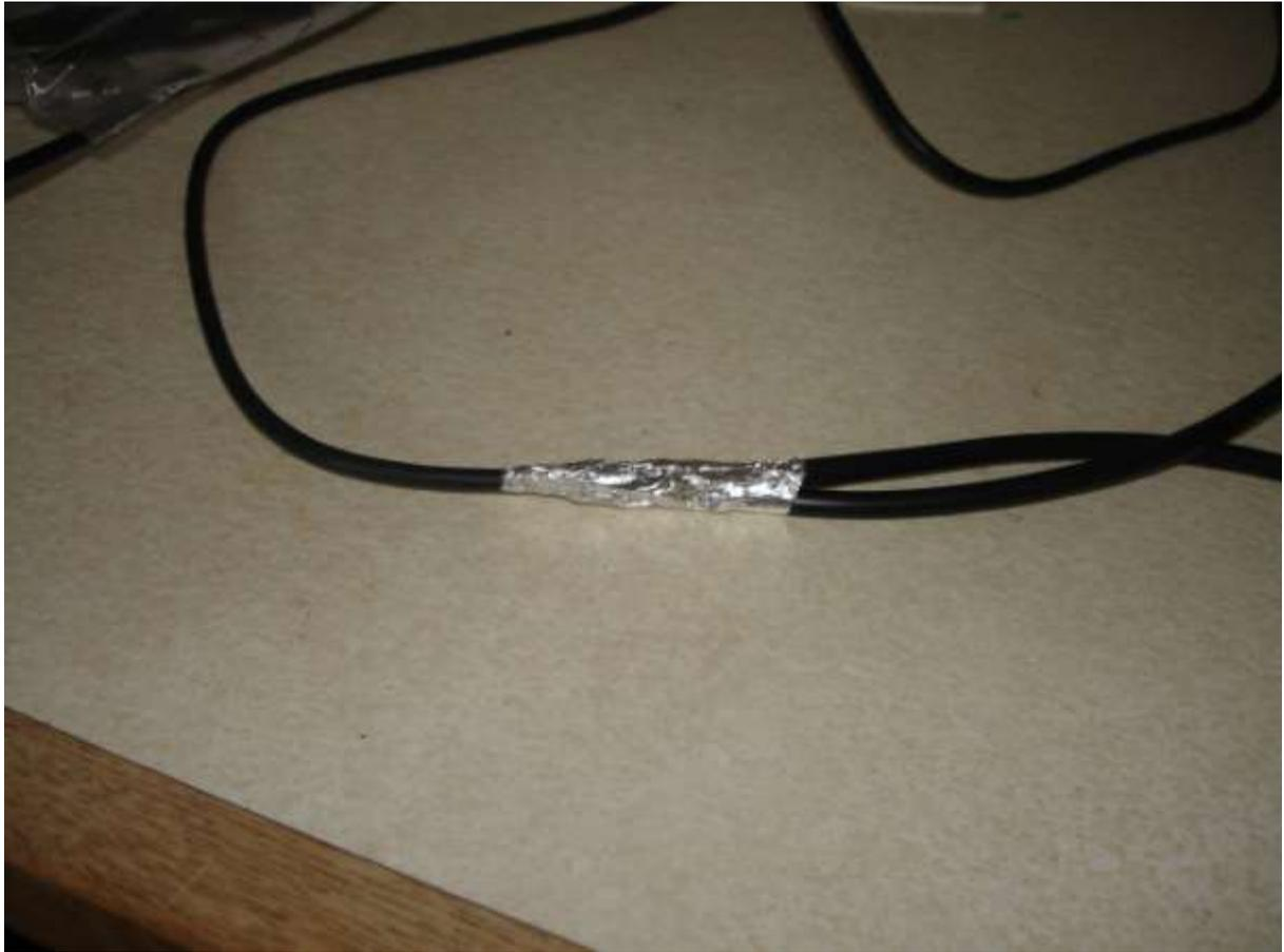
and a piece of tinfoil ensures that the shielding is maintained along the length of the cable.
