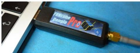
This is simply a small aerial which connects to a special FUNcube USB dongle. Used outdoors, this will receive the signals directly from the satellite and transfer the data to specially developed graphical software running on any Windows laptop.
